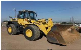
**Wheel loader:** a vehicle that moves rubble from the demolition site to a disposal site.
