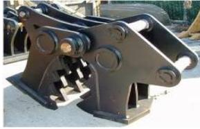
**Demolition attachment:** used to press and crush rubble.
